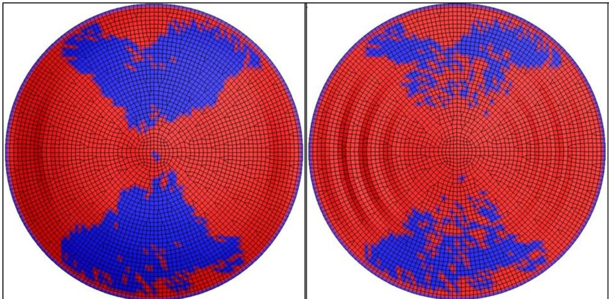
**Figure 6:** Left: Delamination at Peak Deflection Right: Delamination Post Peak Deflection (Red Indicates Delamination, Blue Indicates Tied Nodal Constraint)
