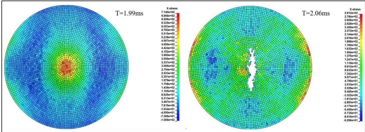
**Figure 5:** Left: Stress in Fiber Direction Just Prior to Failure. Right: Stress in Fiber Direction Just After Failure and Element Degradation/Erosion
