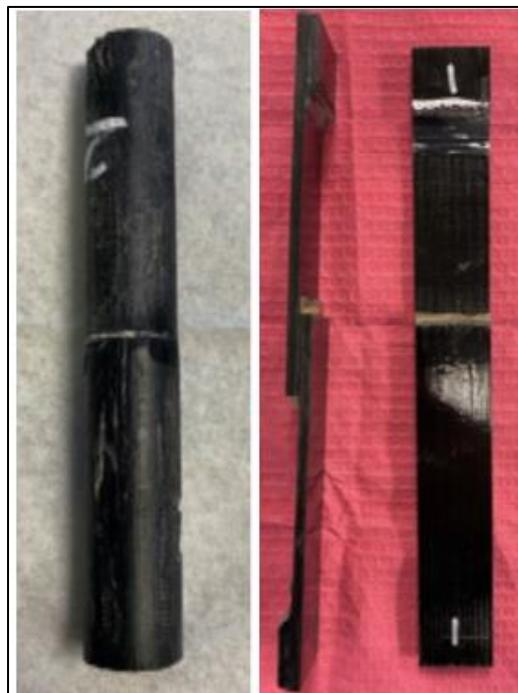
**Figure 3:** (Left) Butt joint specimen used for determining through thickness failure strength (Right) lap shear specimen used for determining shear strength between plies.
