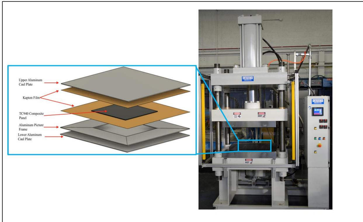
**Figure 1:** Depiction of tool used to manufacture the thermoplastic composite within a heated hydraulic press
