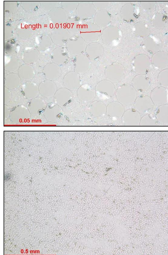
**Figure 4:** (Top) Macro view of distribution of glass fibers and resin rich areas within the composite (Bottom) Close up view of individual glass fibers.
