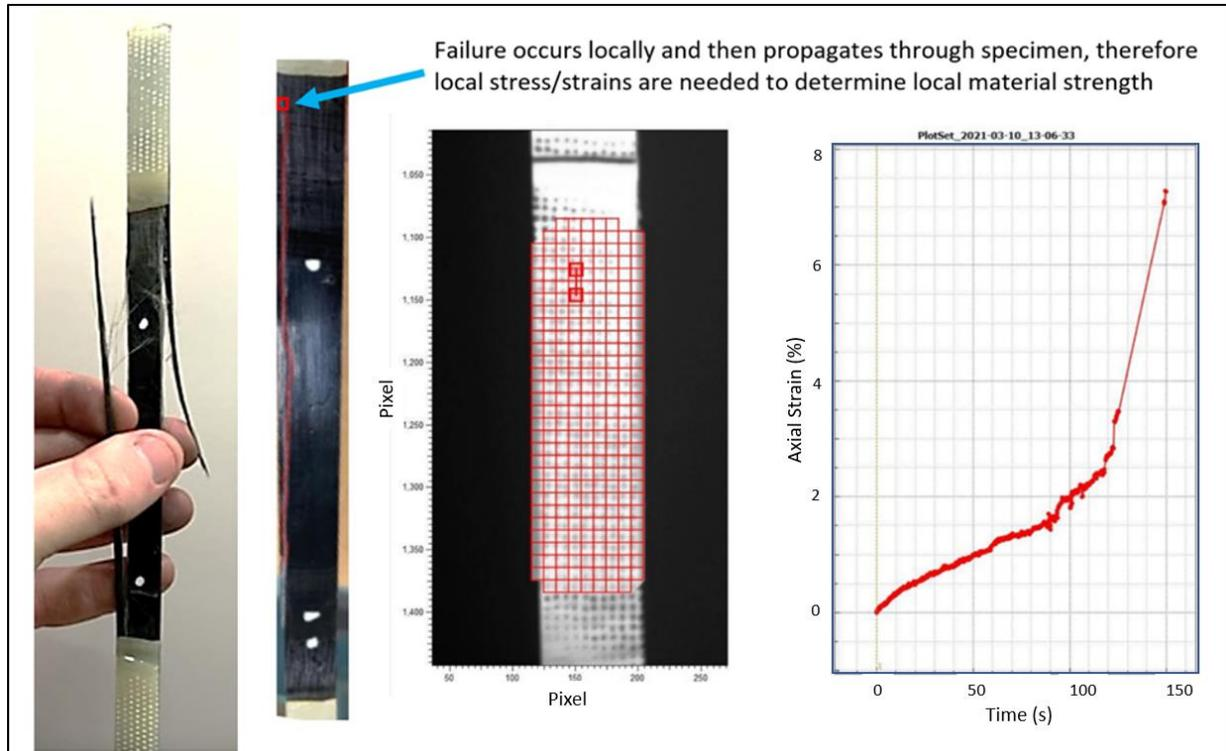
**Figure 2:** Images of unidirectional tensile specimens showing local failure (left) and digital image correlation graph showing local strains within the specimen.
